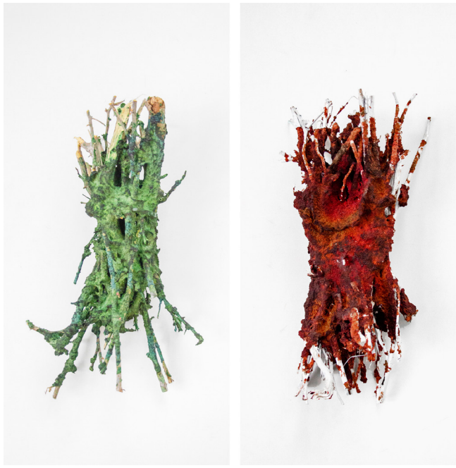
Figure 4. Prototypes showing scavenged twigs and sprayed paper pulp binder.
